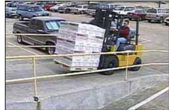
Traveling up ramp with load.
