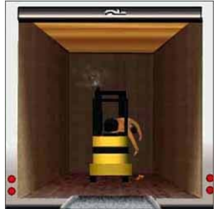
Danger of carbon monoxide poisoning in confined spaces.
