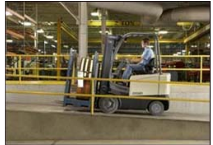
Drive loaded trucks forward going up a ramp.
