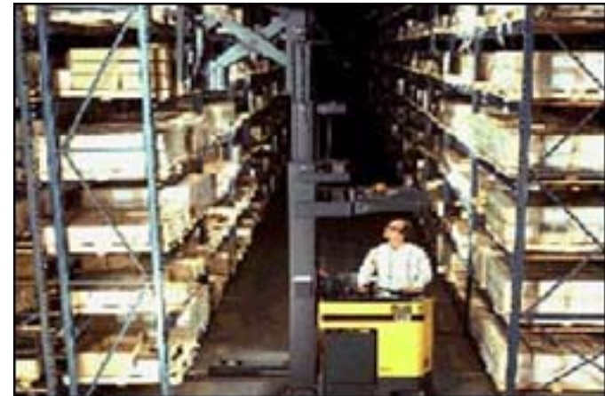
Reach truck with pantograph attachment that scissors forward from the mast to retrieve the pallet.
