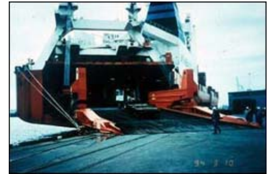
Powered industrial truck engaged in roll-on roll-off (Ro-Ro) operations and subject to 29 CFR 1915.12.
