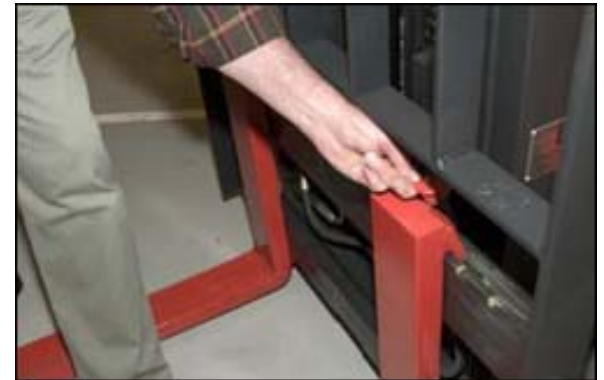
Operator inspecting the top clip retaining pin for the forks.
