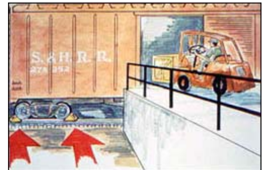
Use positive protection to prevent railroad cars from being moved.
