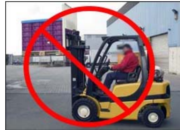
Do not travel with the load elevated.
