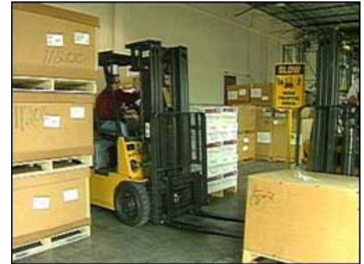
Operator slows down and sounds the horn at cross aisles where vision is obstructed.
