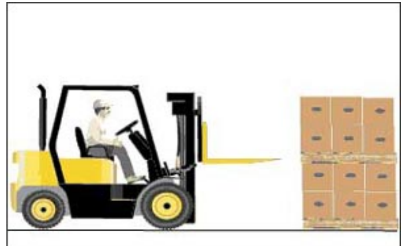
Operator lifts load with the mast vertical.
