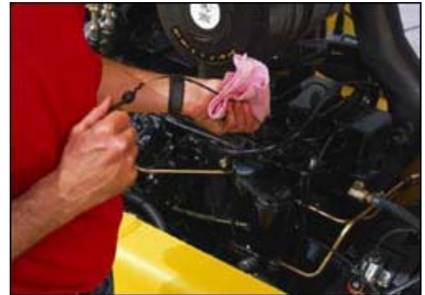
Operator checking fluid levels.
