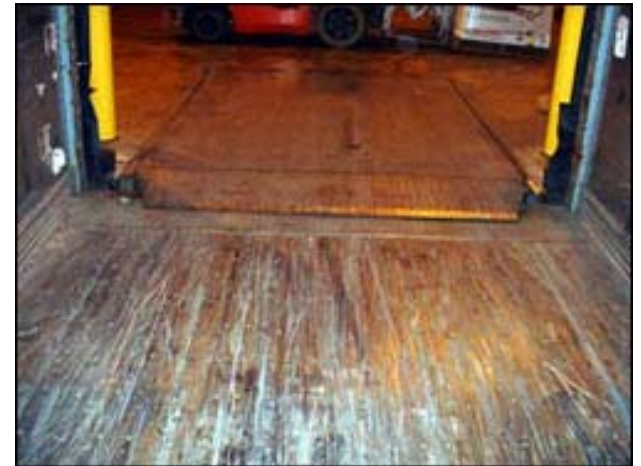
Manual dock plate is secured into position. Always walk and inspect trailer floor before boarding
